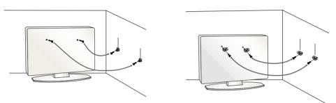
Insert the eye-bolts (or TV brackets and bolts) to tighten the product to the wall as shown in the picture.
